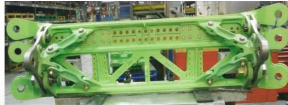
[B737 Rear Spar & Jack Screw Assy.]
